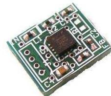
FemtoB uses the Freescale FXOS8700 6DOF sensor - 3-axis accelerometer 3-axis magnetometer
